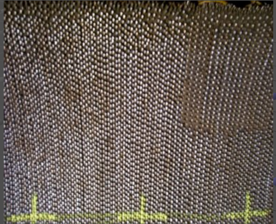
➤ T5 studs on barrel wall
